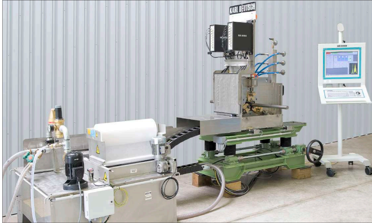
Bar testing system with water filter unit, test table and movable operator panel
