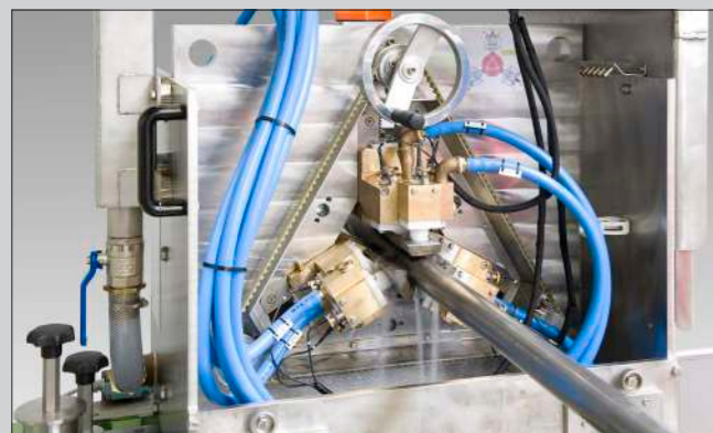
The STP-system works with three probe carriers (couplant wipers and protection housing of the system are dismantled in this picture). Each probe carrier accommodates one probe for normal incidence. Two angle beam probes can also be integrated in each probe carrier for detection of surface-near flaws.
