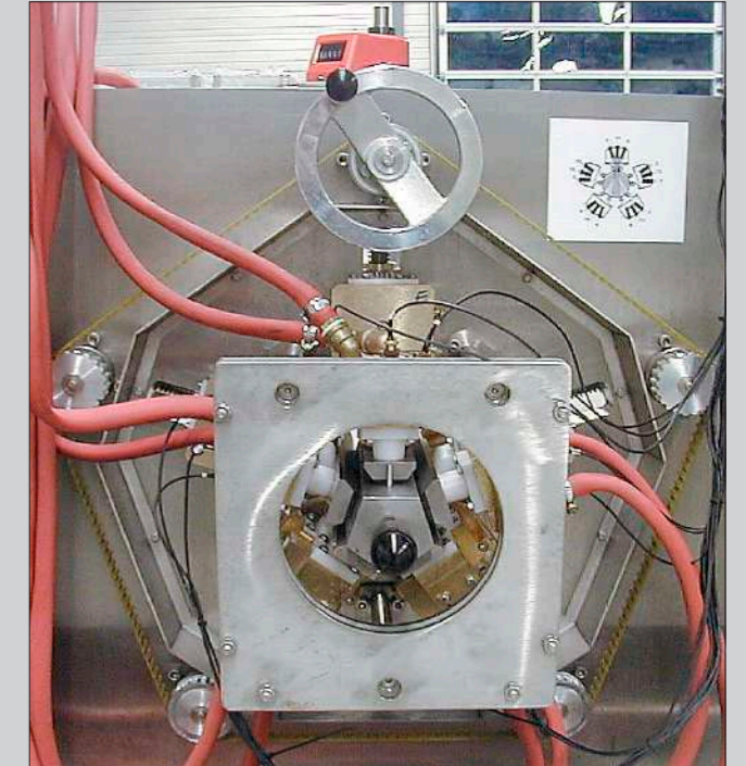
Testing mechanic with 15 probes for round bars (the image shows a pentagonal calibration block)
