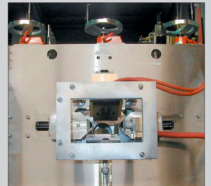
Testing mechanic with 3 dual-element probes for flat profiles
