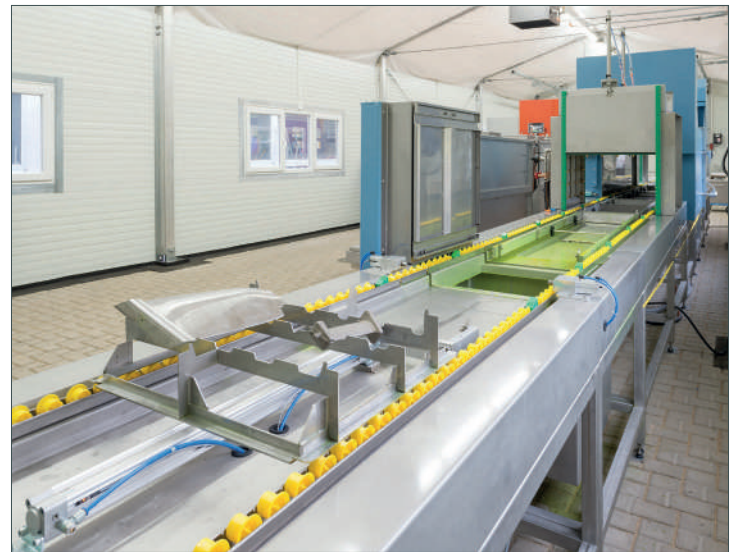
Linear system design with test piece transport by means of a roller conveyor and pneumatic feeding of the workpiece holders. The original parts to be tested are not shown in the picture due to a confidentiality agreement.
