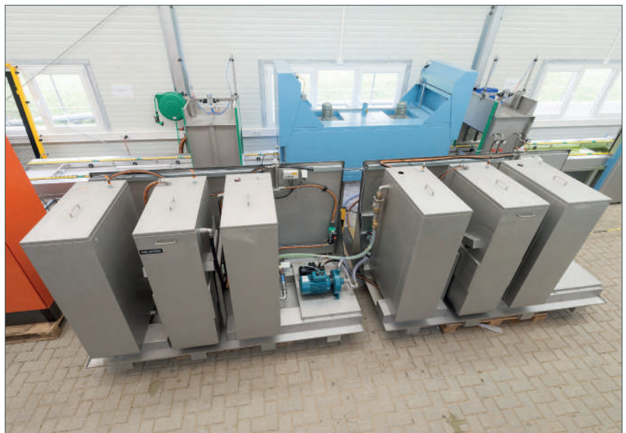
Circuit for the wash water: Regeneration by means of active carbon filtering with a doubled column.
