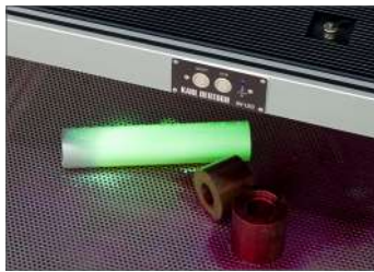
Inspection with the large area lamp under UV light
