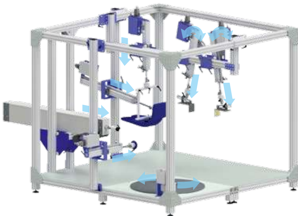
Demonstration of possible movement and load directions of the test axes in a universal test field
