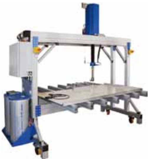
Test rig for 90° peel tests on solar modules
