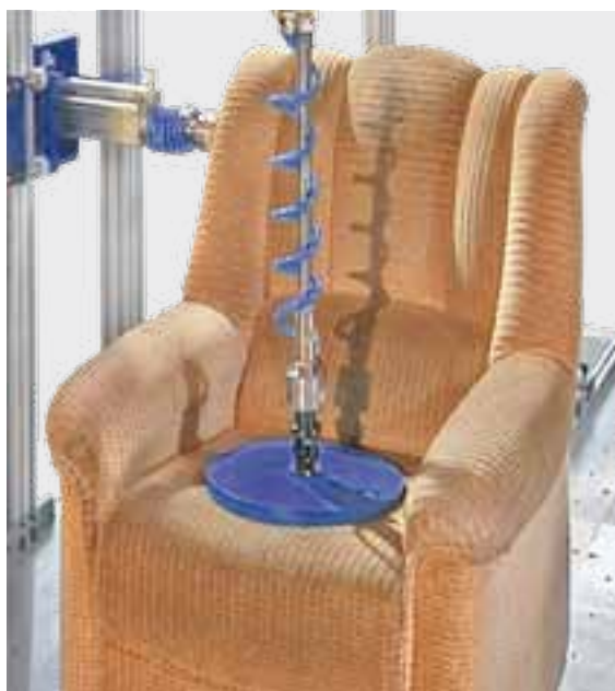
Armchair testing in the universal test field
