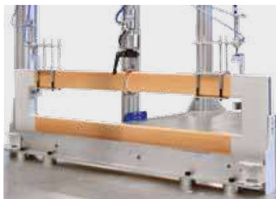
Test of side rails on nursing care beds in the universal test field
